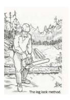
Leg Lock Method – Engage the Chain Brake. Left hand grip on front handle. Arm straight. Rear handle between legs just above knees. Stay on
